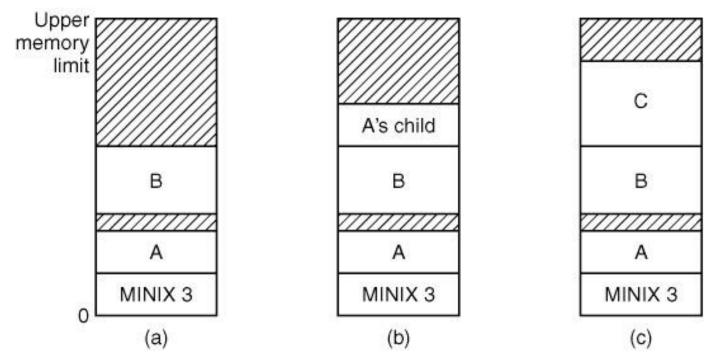
• (a) Originally. (b) After a fork. (c) After the child does an exec.
